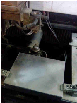
Figure 3.2 AISI A2 Workpiece Material
