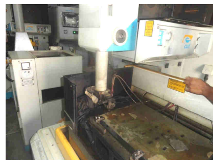
Figure 3.1 WEDM Setup for experimentation
